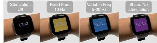
**Figure 5: Modes on the smartwatch (from left to right): Stimulation Off mode with a blank clockface background; Fixed frequency mode at 10 Hz with a yellow background; Varying frequency mode between 5 and 20 Hz with a blue background; Sham mode with no stimulation with a purple background.**
